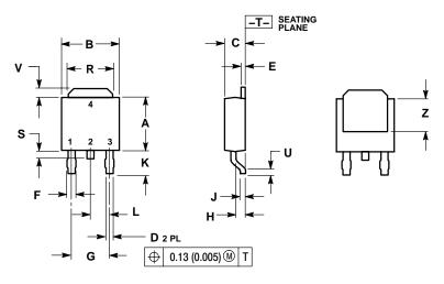
NOTES: 1. DIMENSIONING AND TOLERANCING PER ANSI Y14.5M, 1982. 2. CONTROLLING DIMENSION: INCH.
